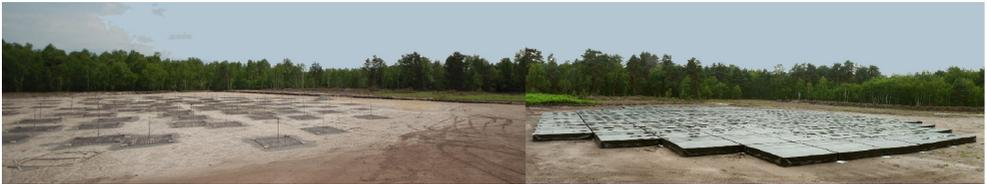
Figure 2.: *The low-frequency (left) and high-frequency (right) LOFAR phased arrays in Nançay.*
