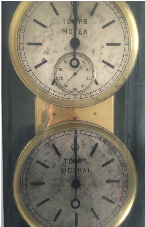
Typical astronomical clock providing Mean solar time & Sidereal time: the Esclanon clock (Paris Observatory, bâtiment Perrault)
