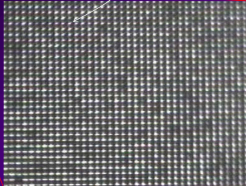
Close-up of a CCD Imaging Array
