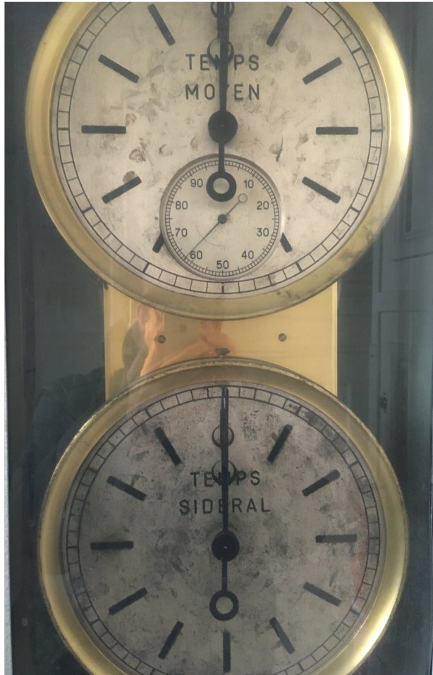
Typical astronomical clock providing Mean solar time & Sidereal time: the Esclangon clock (Paris Observatory, bât Perrault)
