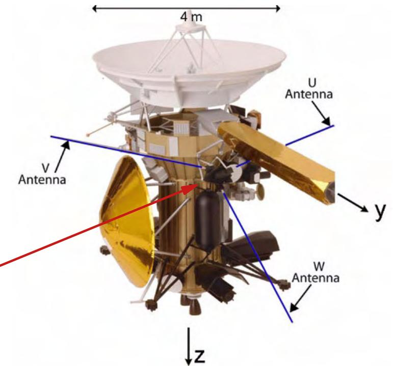
Dust analyser not calibrated for nanodust
