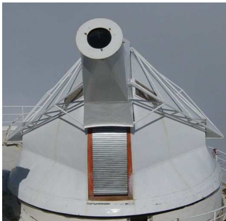
Fig. 5: Mehlretter's ring to avoid heating of the lens holder.
