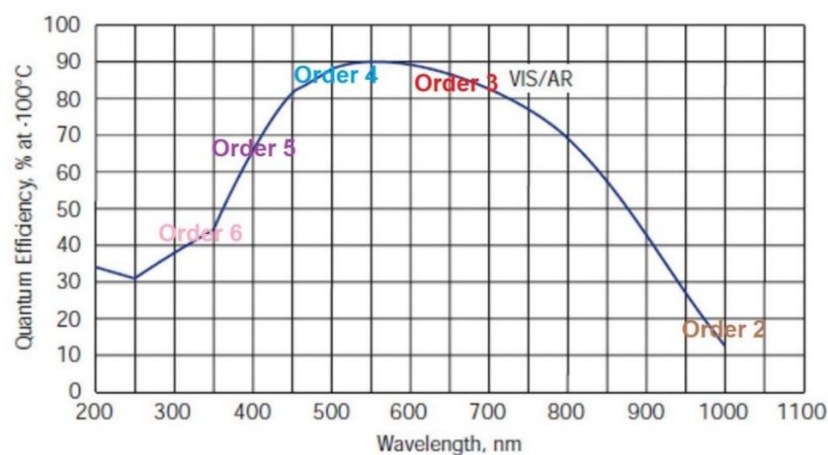
Figure 14. The quantum efficiency of the 2002 back illuminated CCD detector with VIS/AR + Lumogen coating. Call K and H \alpha are respectively observed in orders 5 and 3. H \beta is visible in order 4. Courtesy Paris Observatory.
