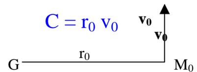
$$\text{Alors } E = 1/2 \mu v_0^2 - K m_1 m_2 / r_0 = 1/2 K m_1 m_2 (e^2 - 1) / p$$
