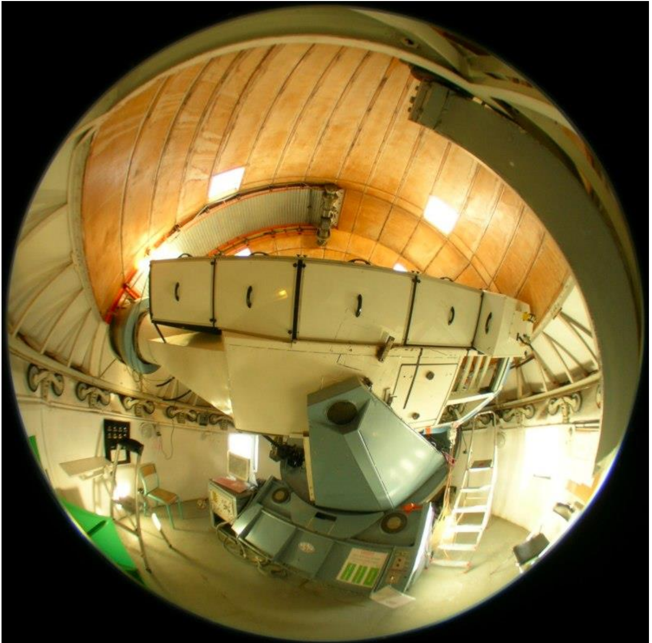
Figure 11: A fish eye view of the 0.5 m / 6.5 m refractor and the 8.0 m focal length spectrograph above (courtesy S. Rondi).
