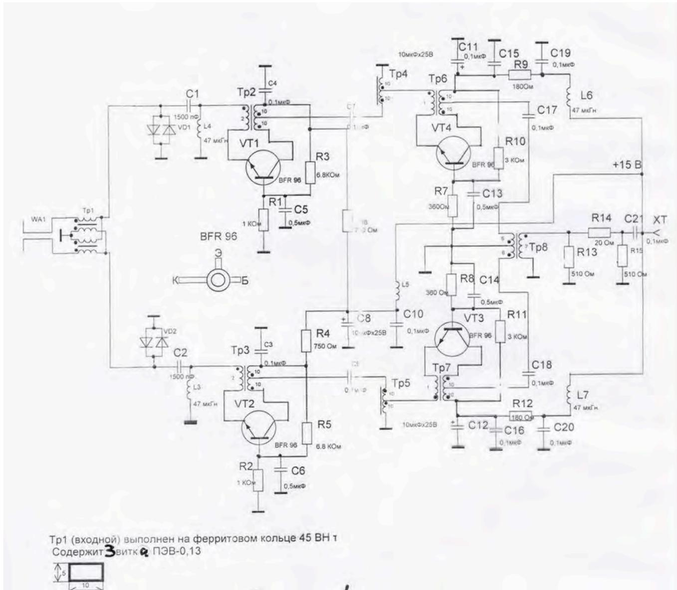
Preamplifier of active antenna element
