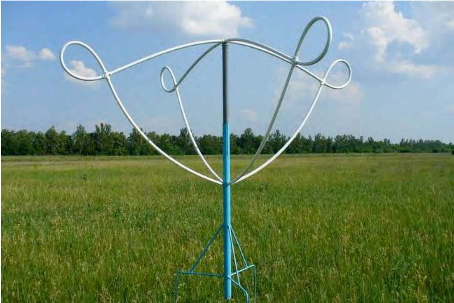
New active antenna element (10-60 MHz,  $k=3\dots 10$  dB)
