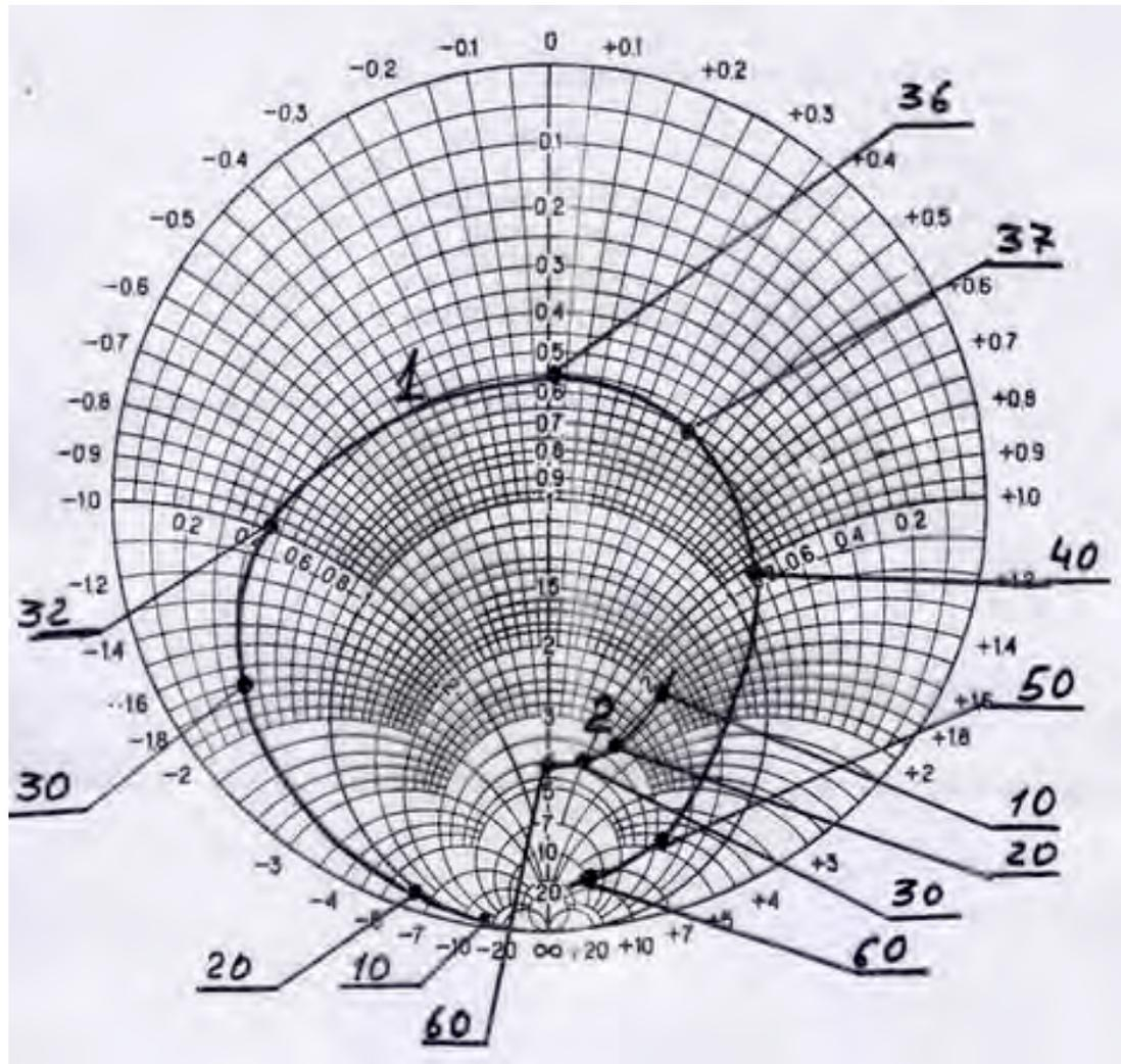
Impedances of antenna element and preamplifier
