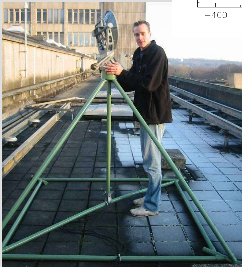
LORUN (4x2 crossed dipoles) (LOFAR @ Radboud University Nijmegen)
